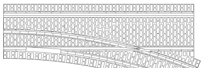
32mm and 16.5mm intersection with 16.5mm gauge track diverting to left/right of inside of 32mm gauge. Fit code 100 rail
