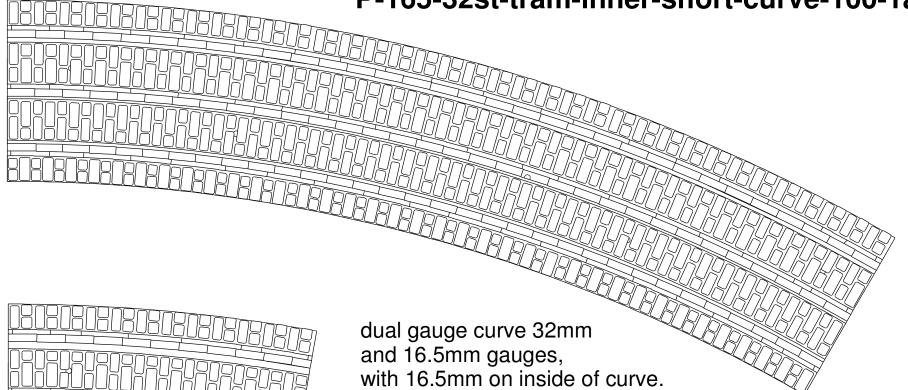
overall angle is 10 deg and 30deg. fit code 100 rail
